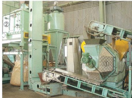
①造粒機/SPM-580 ②冷却機/MPC-1414
